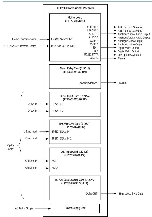
Figure 2.5: TT1260 Signal Connections
